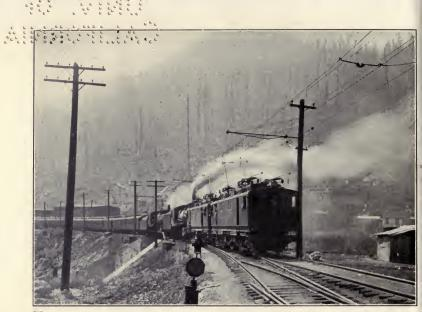
Two triple-phase locomotives of the Great Northern Railway helping a double-header steam train up the grade into the Cascade Tunnel
